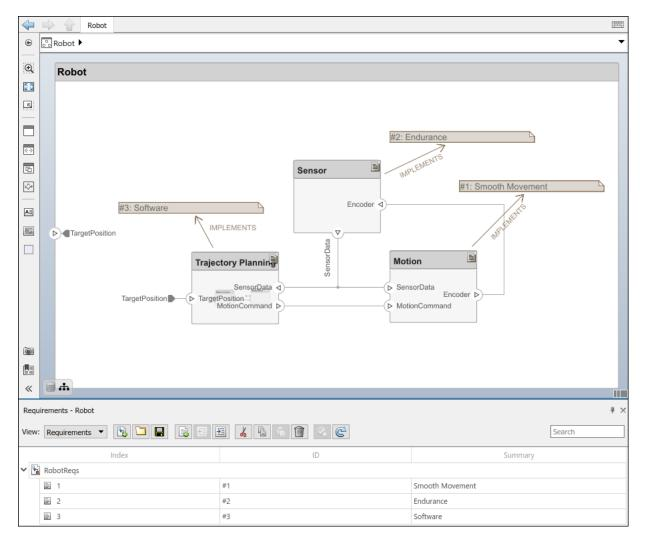
To enhance the traceability of requirements, link requirements to architectural components and ports. When you click a component in the Requirements Perspective, linked requirements are highlighted. Conversely, when you click a requirement, the linked components are shown. To directly create a link, drag a requirement onto a component or a port.
