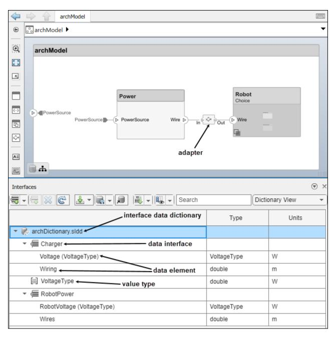
Manage interfaces local to a port using the Interface Editor in Port Interface View.
