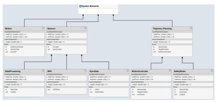
8 Navigate to **Diagram > Architecture Hierarchy** to display unique architecture types and their relationships using composition connections.
