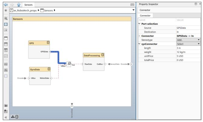
6 Complete the model using the desired property values. Pin the Property Inspector to the editor to keep the Property Inspector visible during this operation.
