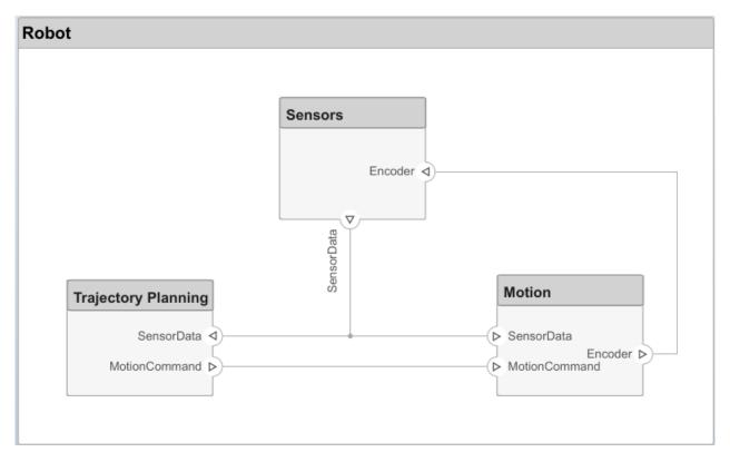
The root level of the architecture model can also have ports that describe the interaction of the system with its environment. In this example, the target position for the robot is provided by a computer external to the robot itself. Represent this relationship with an input port.
