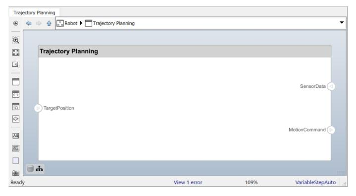
This component first uses the motor position data that is part of the sensordata interface to compute the ideal position and velocity command. It then processes the obstacle distance information in the same interface to condition this motion command according to some safety rules.
