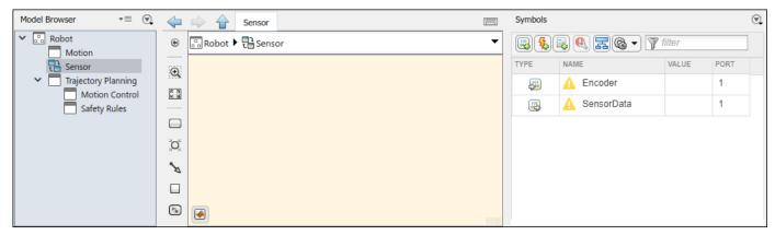
**3** Select the SensorData output and view the interface in the Property Inspector. You can access the interface like a Simulink bus signal.
